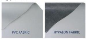
**A. Back of Fabric;** If you can see the inside of the tube, through the valve, Hypalon is a dark grey or black on the inside. PVC is the same colour on both sides.
